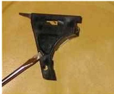
Push the disassembly catch spring down, tilt the frame to the side, and shake. The catch will come out. The spring that held it is just lying loose in the frame at this point. If you only want to get to the trigger, you can skip this step.
