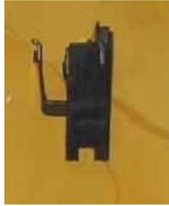
Hook up the spring to the trigger bar, and put it back the way it was. It does not take any force other than to overcome the small spring.
