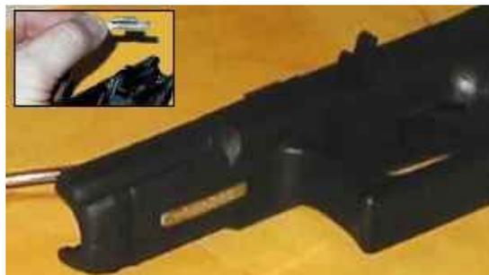
Put the locking block back in the frame, and check that the holes align.
