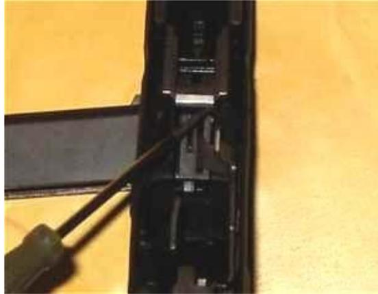
Insert the punch under the ejector in the same way, and gently pry the trigger assembly out of the frame. The impression here is that the whole guts of the gun are coming out, that's as it should be.
