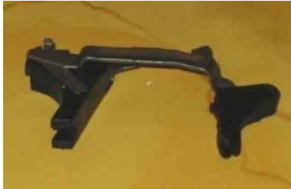
Put the trigger assembly back into the frame, and check that the holes align.
