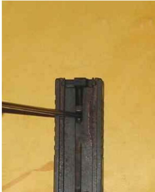
While doing that, slide the back cover of the slide downwards, and pull the firing pin (Glock refers to this part as "the striker", which is probably a better name, as the gun is striker fired, i.e. there is no hammer. I'm going to use the two words interchangeably in this article) and extractor spring that become visible clear to the rear.
