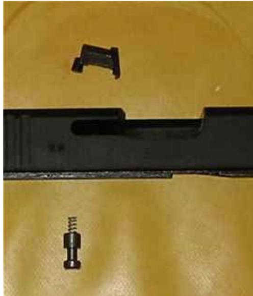
Insert the firing pin assembly and the extractor spring from the rear as shown.
