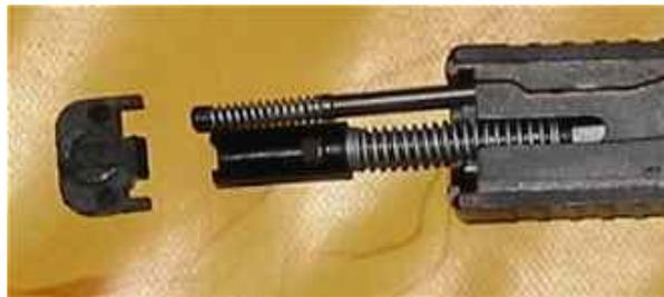
You will have to push down on the firing pin sleeve and the extractor spring pin when the cover reaches them.
