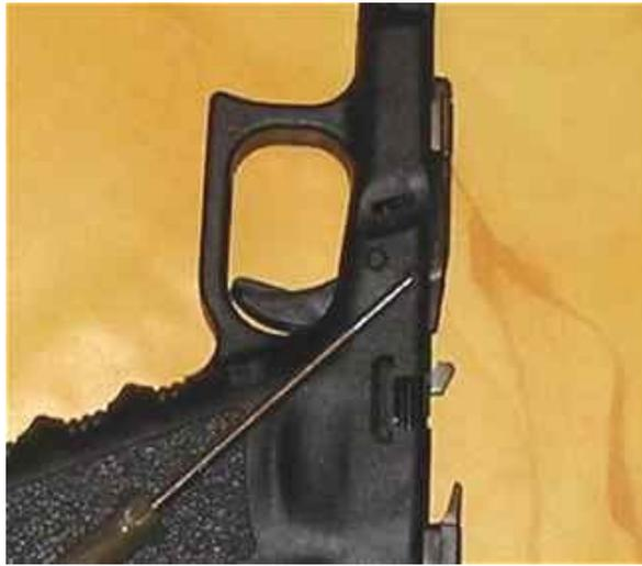
Start pushing the second pin (the larger one that holds the trigger and the slide stop) left to right. The slide stop sits in a recess in the pin, so you may have to tinker with it to get it lined up.
