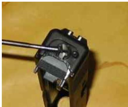
Almost there, time for a function check: Push the firing pin safety in, and shake the slide back and forth. The firing pin should move freely.
