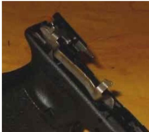
Put the disassembly catch spring back the way it was, push it down with something, and insert the catch from the side (left or right). There is a groove cut into one side of the catch. The catch goes into the frame with this groove facing to the rear. The serrated "ears" (the parts of the catch sticking out of the frame when the gun is assembled) should face down. The part will go in either way, but this is how it should be put in.
