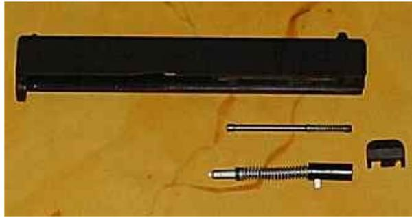
Push the firing pin safety in with your thumb, and wiggle the extractor loose. The firing pin safety is all that is holding the extractor at this point. Once the extractor is loose, lift the firing pin safety out of the slide. Be careful with the small spring that is under it so you don't lose it.
