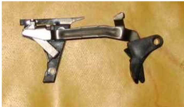
Take a small screwdriver, and locate the point where the connector is fastened. Push it gently to start it out of the plastic block.
