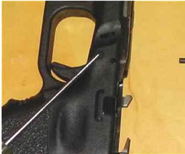
Pull the slide stop out of the frame to the rear and slightly up.
