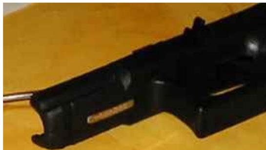
Here's another one that's easier to do than to explain... look down the magazine well. You will see the magazine catch and it's spring. There is a small slot cut in the magazine catch where the spring can be guided out. Use a small screwdriver (pushing the magazine release can help) and do that. The magazine catch will come out of the frame to the right. You can skip this step if you were only interested in the trigger.
