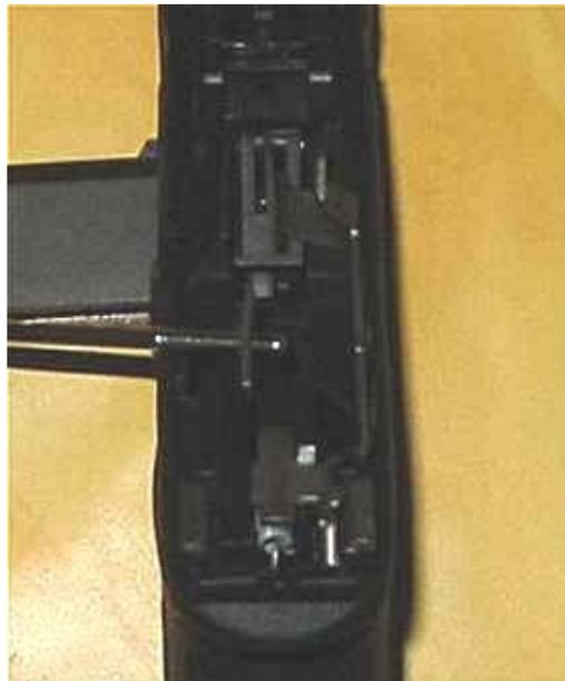
Trigger assembly. Gently twist the trigger bar out of the plastic block that holds it and the ejector. Unhook the spring that connects them. Take a mental note of how it's all hanging together.
