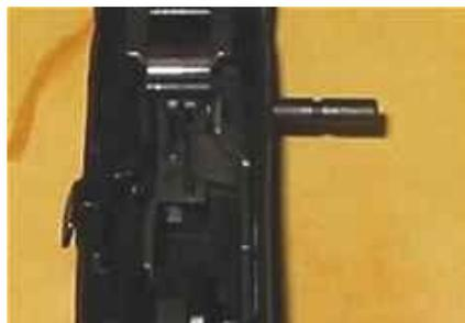
Put the firing pin in its plastic sleeve, and put the firing pin spring back on the firing pin. If you want to cheat, you can stuff the rear end of the sleeve with TP, but it can be done without. Push the spring down with one hand, and put the little plastic retaining things back around the pin using hands two and three ;-). Don't let the spring slip.
