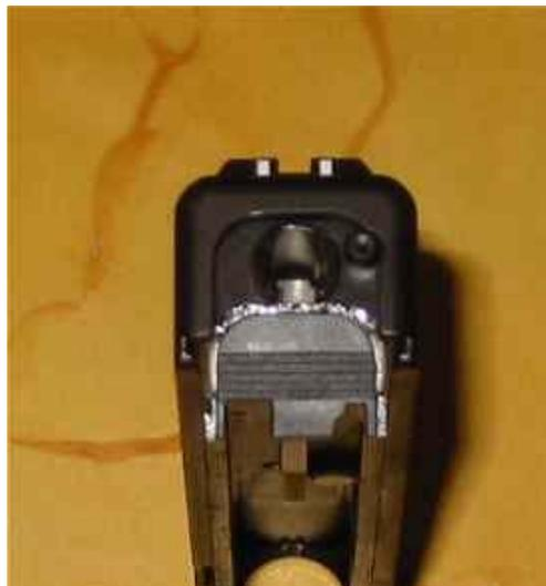
Firing pin and extractor spring. When the cover comes off, there is some spring pressure, but not a whole lot...
